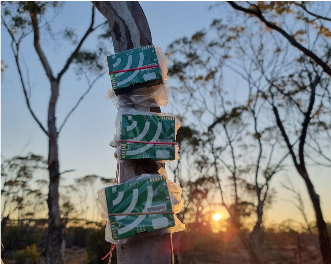
Figure 9. AudioMoths set in triplicate to determine optimal recording parameters for Yookamurra prior to the Microbat Survey (Lachlan McRae/AWC).
